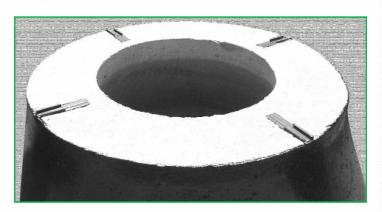
The **A**•LOK BOLT SLOT INSERT is a slotted insert designed to be cast into the conical or slab top section of underground concrete structures for the purpose of anchoring the cast iron frame to the structure. The insert assembly consists of a tough polypropylene shell and a .75 inch square galvanized nut.
