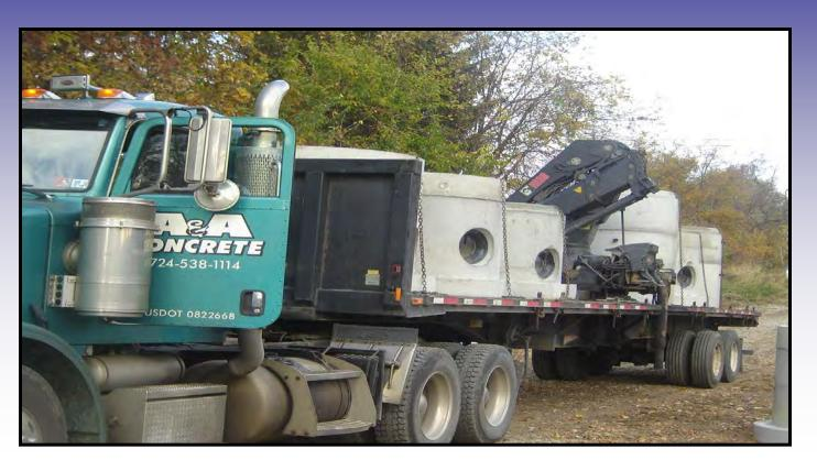
They were also outfitted with our Z•LOK cast-in flexible rubber connectors to create a watertight structure.
