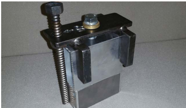
U-Shape Down with 3" Shim Setup 5 9/16" Height
