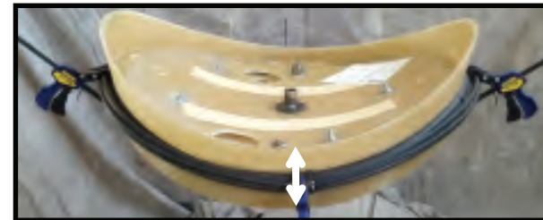
Fig. 2 A-LOK Connector Mounted on Mandrel
