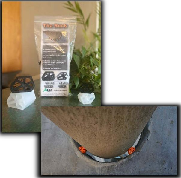
**The ROCK™** is a multi-faceted dimensional spacer engineered to assist with mortar pipe connection. **The ROCK™** is a solution designed as an alternative to using sticks, stones or chunks of concrete or brick as a common practice for supporting and controlling the pipe within the structure opening prior to placing the mortar in the annular space.
